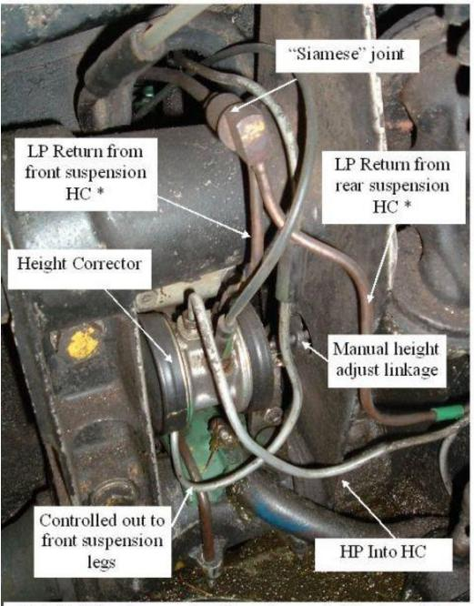
Note that the pipes marked \* are siamesed at the large joint and they both have a wire insert which reduces the internal diameter to a very small amount. This slows down the rate of return to tank and consequently slows the response to the "suspension too high" attitude.
